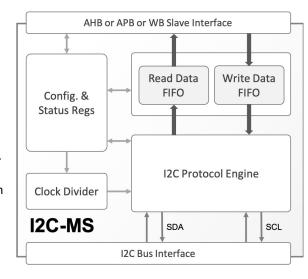
The I2C-MS core is rigorously verified, and silicon-proven. It is available in synthesizable RTL and FPGA netlist forms, and includes everything required for successful implementation, including a sophisticated self-checking testbench, simulation scripts, test vectors, and expected results, synthesis scripts and comprehensive user documentation.
