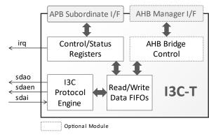
gets. It can be assigned a Dynamic Address by the bus controller or use its legacy I2C static address, it supports Hot Join and is capable of generating In-Band Interrupts when directed by the host to do so.
