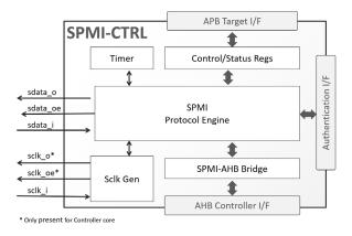
allows integration with application specific authentication logic, which can be reduced to just hardwiring the authentication response data. The core uses separate clocks for its APB and AHB bus interfaces, and a separate reference clock source for its internal timer. Clocks are independent to each other, with clean clock domain crossing boundaries, and the only requirement is that the AMBA interface clocks have a frequency larger or equal to the maximum SPMI clock frequency.
