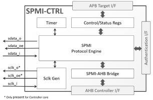
application specific authentication logic, which can be reduced to just hardwiring the authentication response data. The core uses separate clocks for its APB and AHB bus interfaces, and a separate reference clock source for its internal timer. Clocks are independent to each other, with clean clock domain crossing boundaries, and the only requirement is that the AMBA interface clocks have a frequency larger or equal to the maximum SPMI clock frequency.
