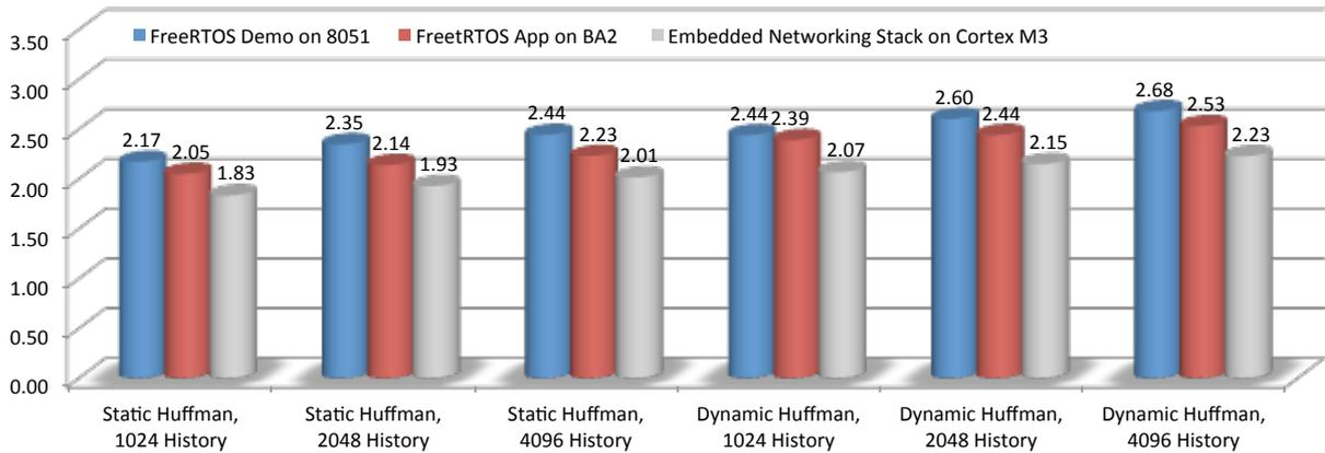
**Figure 3:** Compression Ratio for the image of InterNiche's demo of embTCP and embHTTP.
