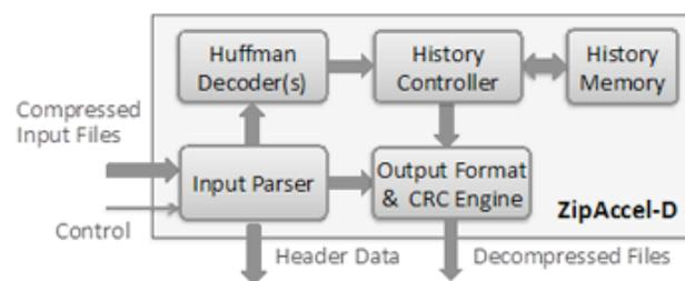
**Figure 2:** Hardware lossless data decompression engine; Huffman decoding type and History size are parameterized.
