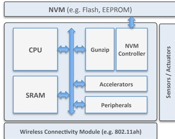
**Figure 1:** System architecture for Code Shadowing with Decompression.
