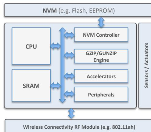
**Figure 4:** IoT architecture with integrated hardware data compression.
