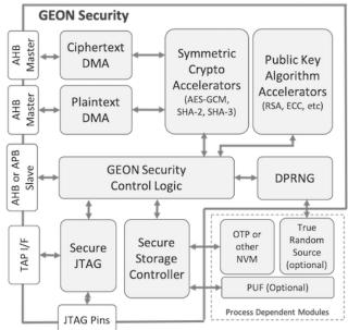
These modules work together and share resources to reduce the chip area and overhead required for complete SoC security. For example, if multiple modules need AES-GCM encryption, the GEON Platform implements and shares a single AES-GCM function to save area in the security block.
