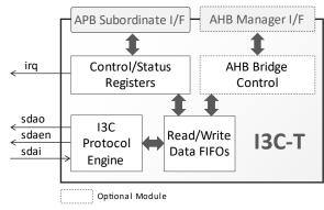
gets. It can be assigned a Dynamic Address by the bus controller or use its legacy I2C static address, it supports Hot Join and is capable of generating In-Band Interrupts when directed by the host to do so.
