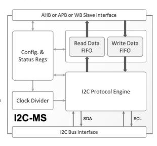
The I2C-MS core is rigorously verified, and silicon-proven. It is available in synthesizable RTL and FPGA netlist forms, and includes everything required for successful implementation, including a sophisticated self-checking testbench, simulation scripts, test vectors, and expected results, synthesis scripts and comprehensive user documentation.
