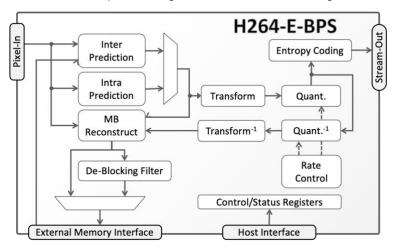
domain, is independent from the external memory type and memory controller, and is tolerant to large latencies. The core is optionally delivered with a raster-to-block converter, and wrappers for AMBA® AHB, AXI, or AXI-Streaming buses are available.
