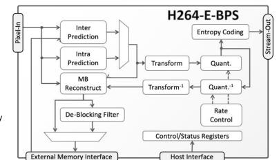
domain, is independent from the external memory type and memory controller, and is tolerant to large latencies. The core is optionally delivered with a raster-to-block converter, and wrappers for AMBA® AHB, AXI, or AXI-Streaming buses are available.
