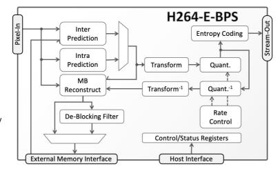
domain, is independent from the external memory type and memory controller, and is tolerant to large latencies. The core is optionally delivered with a raster-to-block converter, and wrappers for AMBA® AHB, AXI, or AXI-Streaming buses are available.
