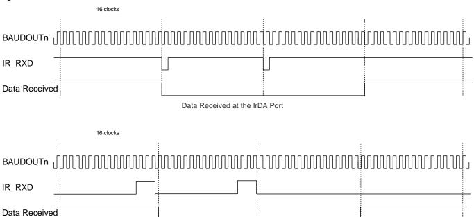
Data Received at the IrDA Port using a positive pulse
