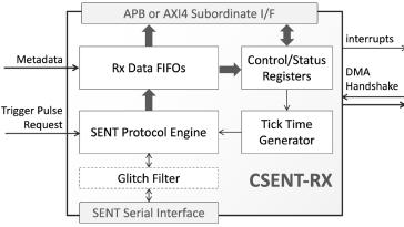
The core provides a glitch filter on the serial data input and has data mapping functionality on
