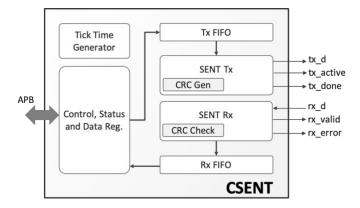
interrupt signals facilitates interrupt-based operation. The core allows for Transmitter operation without requiring any external programming or control. The reset values for all its control registers are defined at synthesis time, and at run time the system only needs to write sensor data to the core.
