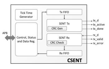
interrupt-based operation. The core allows for Transmitter operation without requiring any external programming or control. The reset values for all its control registers are defined at synthesis time, and at run time the system only needs to write sensor data to the core.
