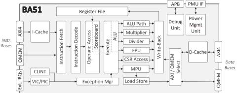
Furthermore, the BA51 supports software and timer interrupts and up to 64 external interrupt lines. It features a remarkably low interrupt response time, which makes the core ideal for real time control applications. The time elapsed from when an external interrupt is asserted until the first instruction in the resolved interrupt handler can be issued is just 4 clock cycles.
