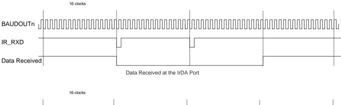
Data Received at the IrDA Port using a positive pulse
