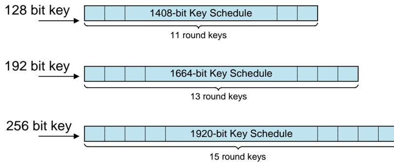
**Figure 3.** Encryption Key lengths and resulting Round Keys
