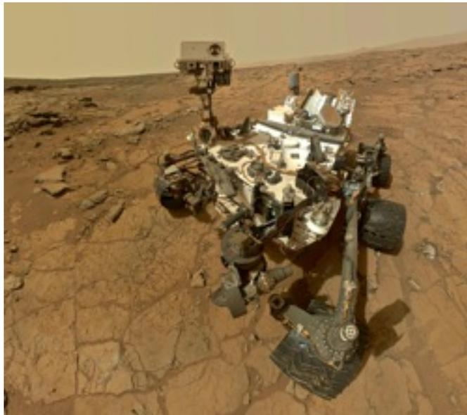
*A selfie taken by Curiosity Mars Rover's mast camera and compressed for transmission by the JPEG core available from CAST. Image Courtesy of [NASA/JPL-Caltech/MSSS](#)*
